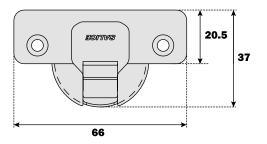
Constant "L" value of 0.7 mm (it does not change during side adjustment).
