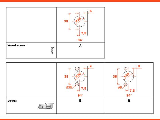
Use this table to identify the available drillings and fixings. Fill the third position of the hinge code number with the letter or the number corresponding to your choice. I.e.: C6\_7C99.
