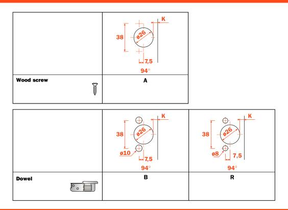
Use this table to identify the available drillings and fixings. Fill the third position of the hinge code number with the letter or the number **corresponding to your choice. I.e.: C4\_7A99.** Fill this position with the chosen letter or number.
