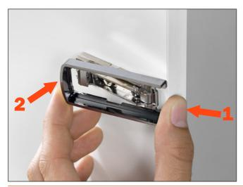
Clip the hinge onto the mounting plate.
