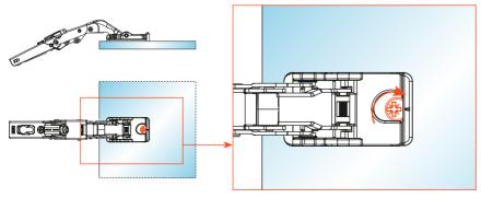
**3)** Rotate the fixing cam with a #2 Pozi screw driver.
