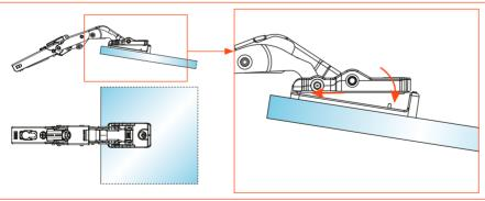
**2)** Locate the hinge onto the plate when it is bonded to the door.
