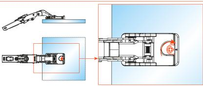
3) Rotate the fixing cam.
