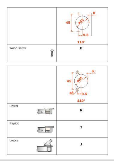
Use this table to identify the available attachment options to the door. Fill the third position of the hinge code number with the letter or the number corresponding to your choice. I.e.: C7\_6AE9.
