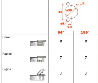
Use this table to identify the available attachment options to the door. Fill the third position of the hinge code number with the letter or the number corresponding to your choice. I.e.: C2\_BAE9.
