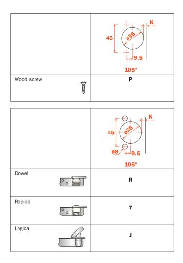
Use this table to identify the available attachment options to the door. Fill the third position of the hinge code number with the letter or the number corresponding to your choice. I.e.: C1\_6AE9.
