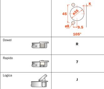
Use this table to identify the available attachment options to the door. Fill the third position of the hinge code number with the letter or the number corresponding to your choice. I.e.: C1\_6AE9.
