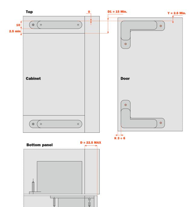
Workings on the top and the bottom panel for the application of the hinge.
