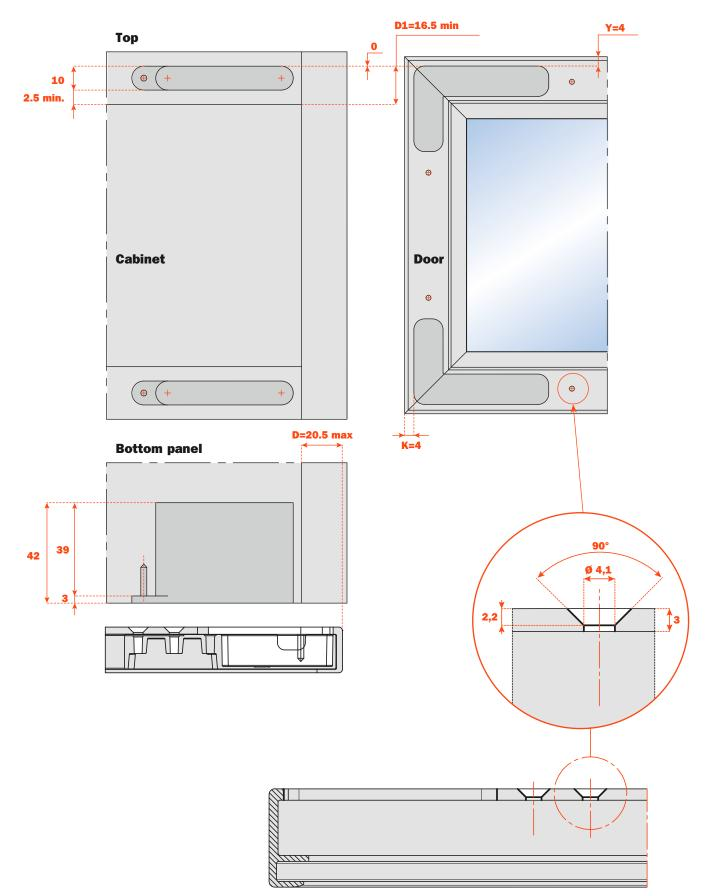
Workings on the top and the bottom panel for the application of the hinge.
