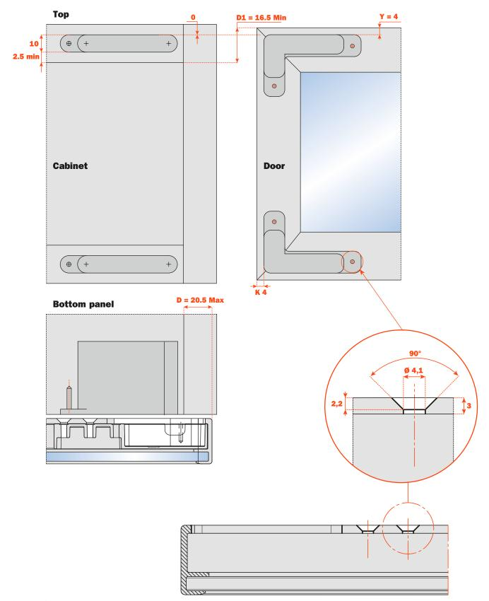
Workings on the top and the bottom panel for the application of the hinge.
