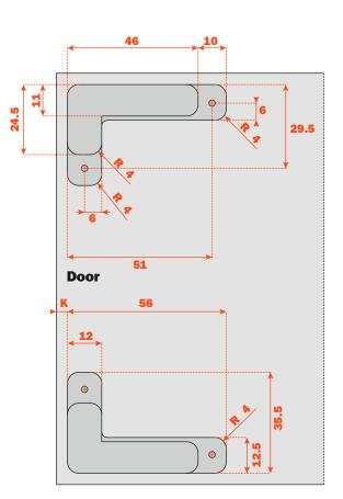
Workings on the frame DEL6LP300\_ and use of the corner connectors DEL6BSFV02.
