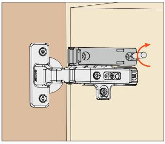
It is possible to reduce or increase the decelerating effect by turning the screw indicated.
