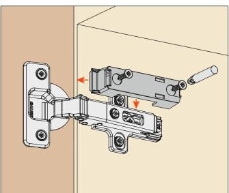
Insert the Smove piston assembly, sliding it in the direction indicated by the arrow.
