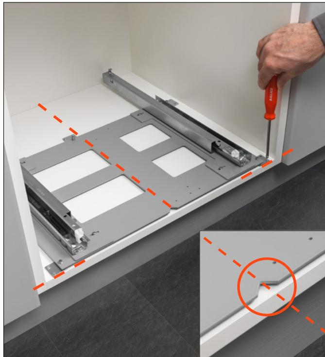
Screw-fix the feet with the screws provided ( $\varnothing$  4 x 18 mm).
