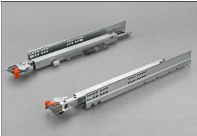
**Full-extension runner system fixed to the drawer by locating pin. The Push self-opening system for handle-less drawers is fully integrated into the runner. A slight pressure on the drawer frontal is sufficient for the drawer to self-open. The Smooth decelerated closing action is also fully integrated into the runner.**
